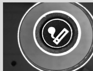
点烟器印刷缺陷检测
