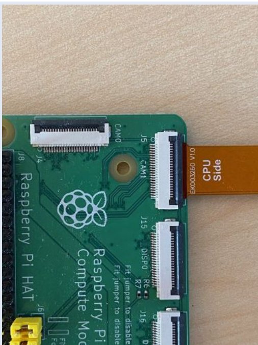
Connect the cable to the CAM1 socket and watch out for the cable orientation
