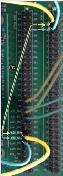
I2C cable bridge to the CAM1 socket.
