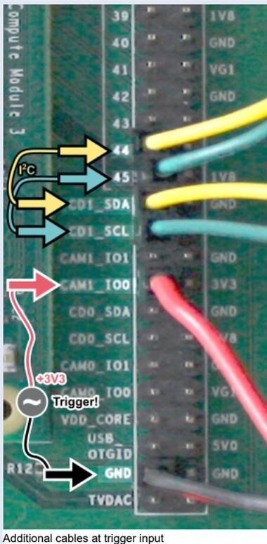
Additional cables at trigger input
