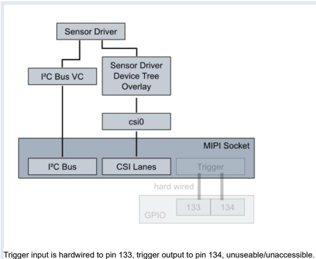
Trigger input is hardwired to pin 133, trigger output to pin 134, unuseable/unaccessible.
