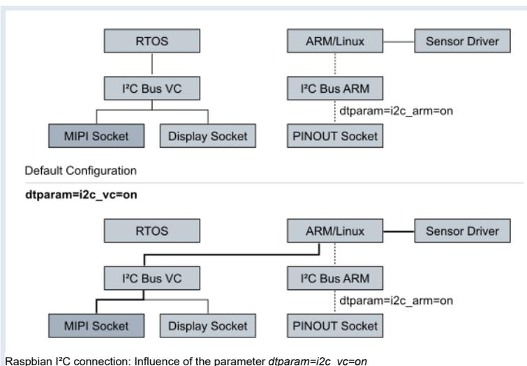
Raspbian I<sup>2</sup>C connection: Influence of the parameter `dtparam=i2c_vc=on`
