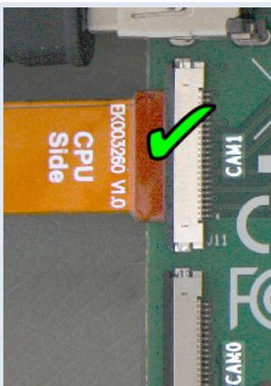
Connect the cable to the **CAM1** socket and watch out for the cable orientation
