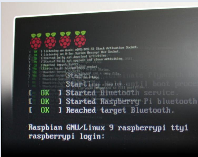
Raspbian showing login screen (user is usually *pi* with password *raspberrypi*)
