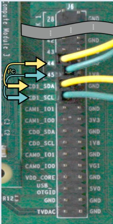
At the J6 connector: I<sup>2</sup>C cable bridge to the CAM1 socket.
