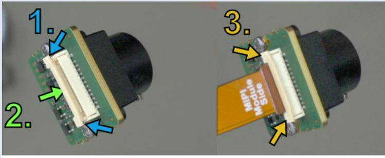
Open the MIPI module socket, put in the cable, close the MIPI module socket
