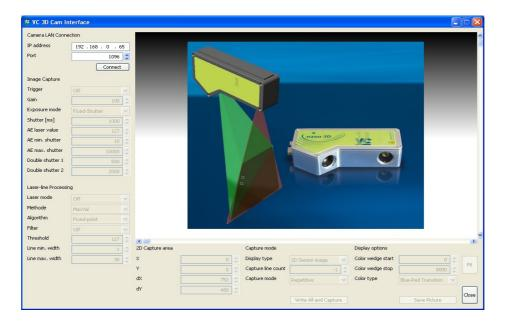
2) After a successful connection to the scanner camera, the tool reads all camera setting parameters.
