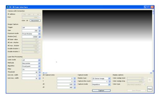
3) Choose Lasermode "ON" and Display Type "2D Sensor image". Then press "Capture". You will get an live image of the sensor scene. Please adjust shutter time sensor position for a stable detection image. Stop the capture mode in order to change the parameters.
