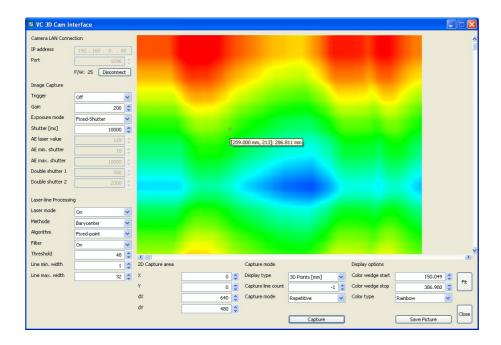
5) Place the cursor inside the transferred image in order to get additional information like position and brightness (2D image) or attitude (3D image) at this position.
