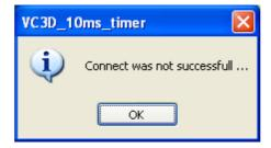
Please check the hardware connection to the camera. You have to use a cross over cable, if you connect the camera directly to the PC. Make sure, that the IP address and port is correct and the camera software is running.
